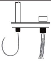
2.Assemble the flexible hoses on the bottom of faucet body.
