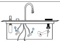
11.Connect the cold and hot water pipe with the kitchen water inlet holes. The inlet pipe of the cup washer can be directly connected to the kitchen inlet or connected to the cold water inlet of the faucet with a three-way angle valve according to the actual situation.
