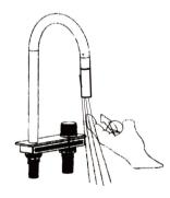
2. When there are impurities to make water flow small, remove the head of the shower frother, cleaning the frother. Just put it back on.
