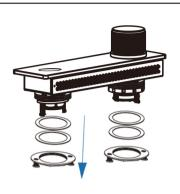
1.Rotary plastic washers and metal washers, remove them from the tooth tube.
