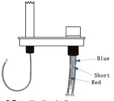
3.Pay attention to the installation position of hot and cold water pipes.
