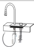
6. Fix the plastic washers and metal washers removed in the first step to the corresponding positions with screws.
