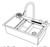
12.Install other accessories like cutting board, small sink and dryer, test them if they are fitting and moving well. Meanwhile test the faucet to see if it is working well.
