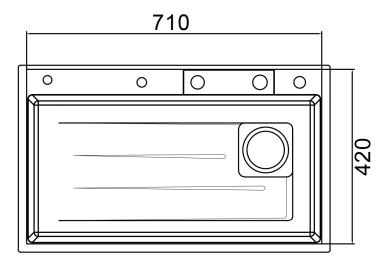
Measure the kitchen countertop to ensure that there is enough space left, and then open the hole according to the figure above.
