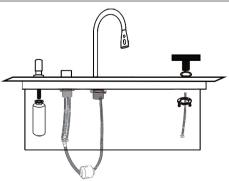
10.Install the dispenser, and cup washer on the sink then put the whole set of sink on the counter top.
